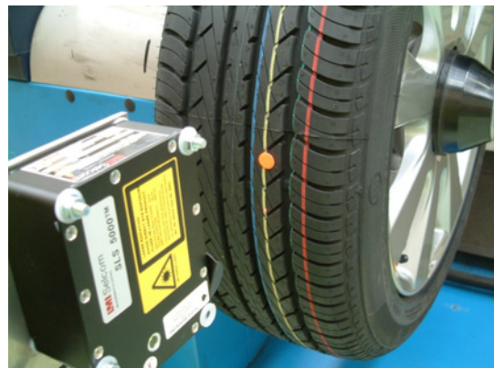
2) Laser sensor mounted on a tripod with "Top of tire" marker
