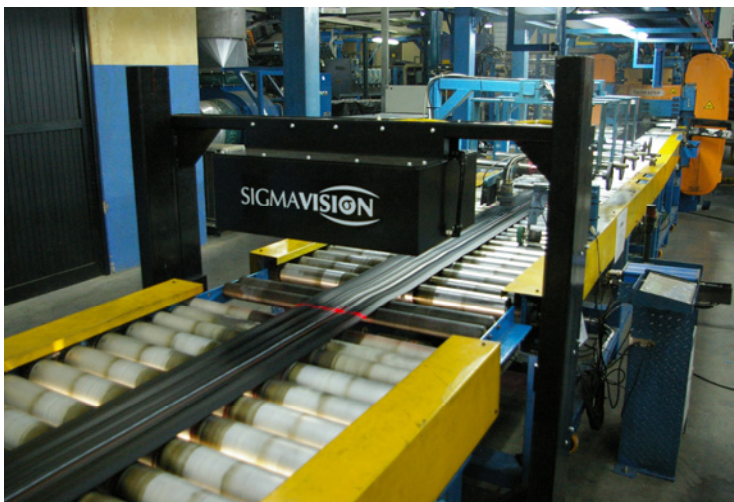
1) Frame mounted on the extrusion line
