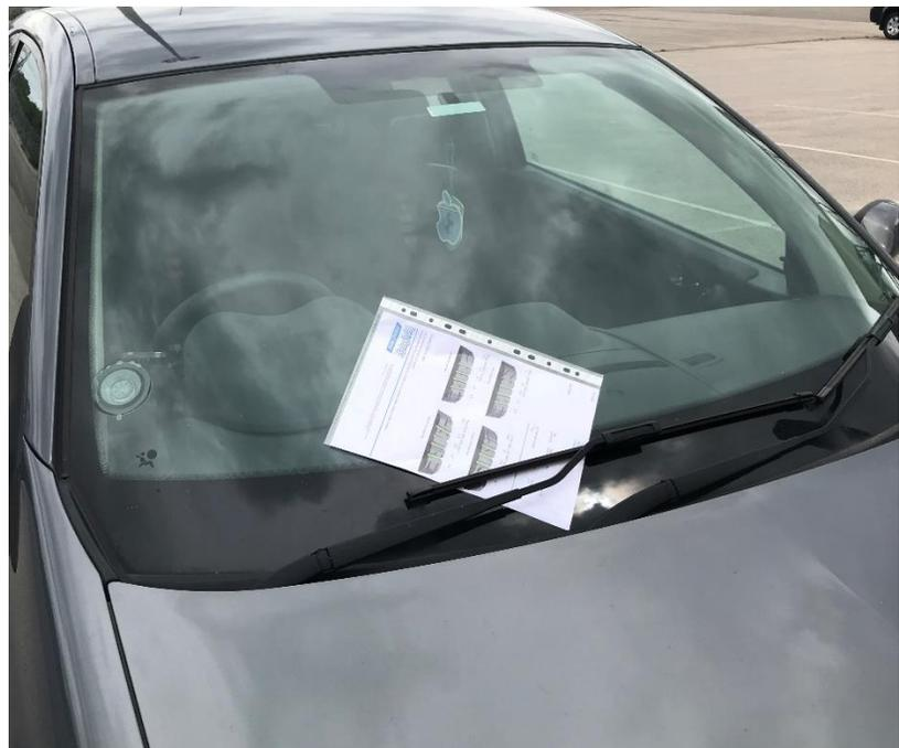
The TreadReader Report contains colour-coded 3D tyre scans to quickly reveal tread depths in relation to the legal minimum. The parameters can be customised, but are typically coded green for >3mm, amber for between 3mm and 1.6mm, then red for tread depths <1.6mm. Uneven wear is also quickly discernable, and photographs in the report are used to show any other anomalies, such as cuts or bulges.
